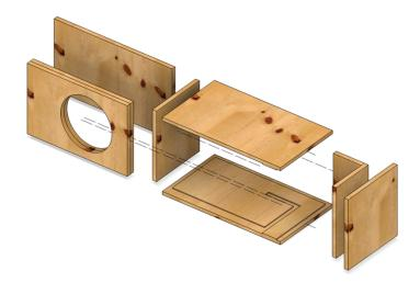
2. If pieces need sanding to fit together properly, sand the necessary edges until they fit snugly.
