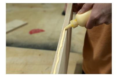
5. Once each piece is glued, clamp it to the adjacent pieces. A tight fit will ensure the highest sound quality. The glue has a few minutes to be fitted together before the bonding process starts.
