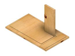
4. Draw a thin, continuous line of glue across the surface of the wood where the two pieces will connect. Only apply glue to the pieces immediately being put together since it dries quickly.
