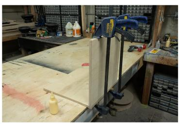
6. While the wood is clamped together, nail or screw the pieces together.
